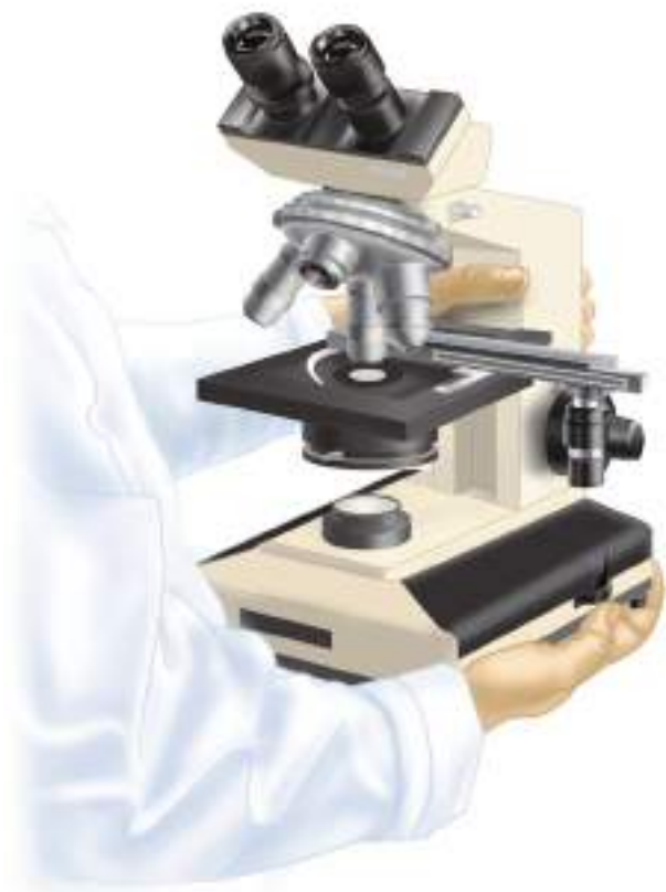
Figure 2.2 The microscope should be held firmly with both hands while being carried.
