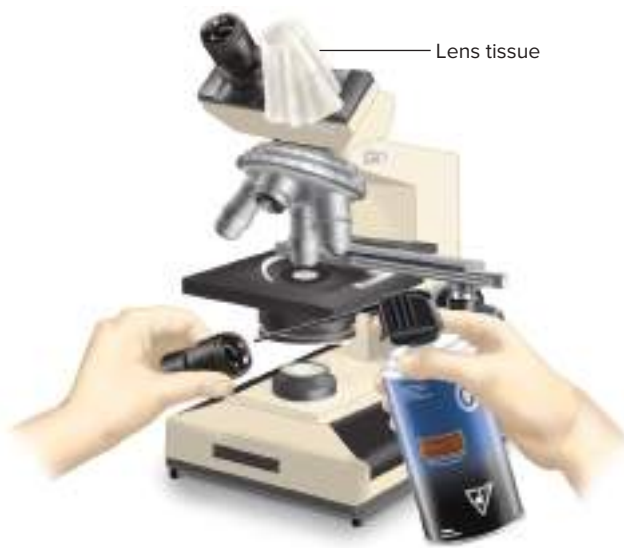
Figure 2.3 When oculars are removed for cleaning, cover the ocular opening with lens tissue. A blast from an air syringe or gas canister removes dust and lint.
